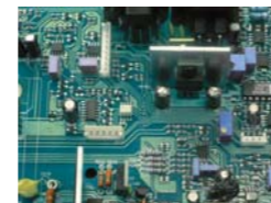
Digital Amplifier main circuit. SMD components. Tropicalized printed circuit boards, for use in salty or extremely humid environments.
