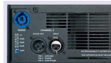
Nominal gain can be adjusted at the back panel with micro-switches (1V, 32 dB, 26 dB, 24 dB)
